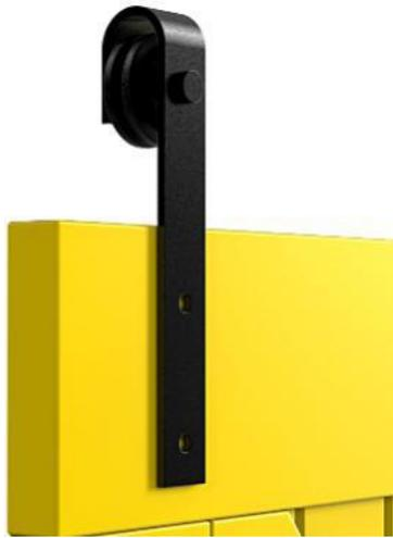
1. Place the hanger on one side of the door. The distance between the top edge of the door and the top hole of the hanger should be 1.6 inches. Mark the position of the holes with a pencil.
